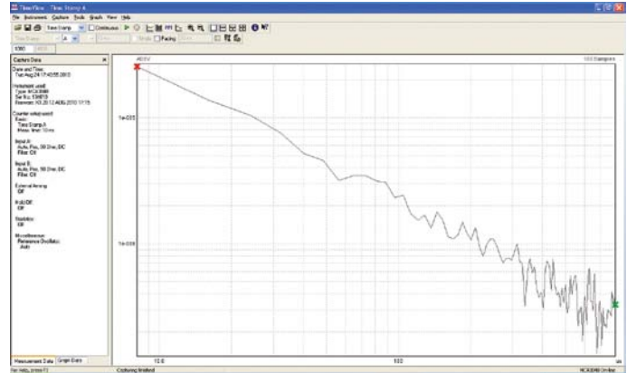
Figure 2. A TimeView™ plot of ADEV vs t for an OCXO.
